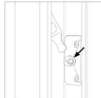
When closed, the sash is held in position by the sash support which can be adjusted to avoid the sash from sagging.
