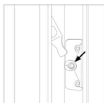
When closed, the sash is held in position by the sash support which can be adjusted to avoid the sash from sagging.
