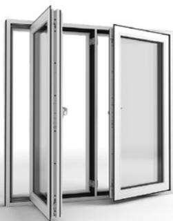
Frame with build-in "easy-clean hinge". windows has the advantage, that window cleaning may be done from inside. Hinges are hidden in the groove and has built-in adjustable friction. With the side mounted fitting, the frame may be opened 90° producing an opening of around 10 cm at the back edge of the frame - enough to reach out and clean the outer face.
