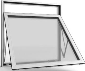
With the top swing ironmongery, the window sash can be pushed out and turned around 170° outside the frame, so the outside of the glass can be cleaned from the inside.
